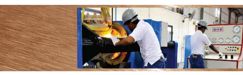
Shell Test, Pneumatic Test, Seat Test can be carried out. Testing Valve size ranging from 2' to 24 " & #150, #300, #600 and #900 can be carried out. Valve testing in horizontal and vertical position.
